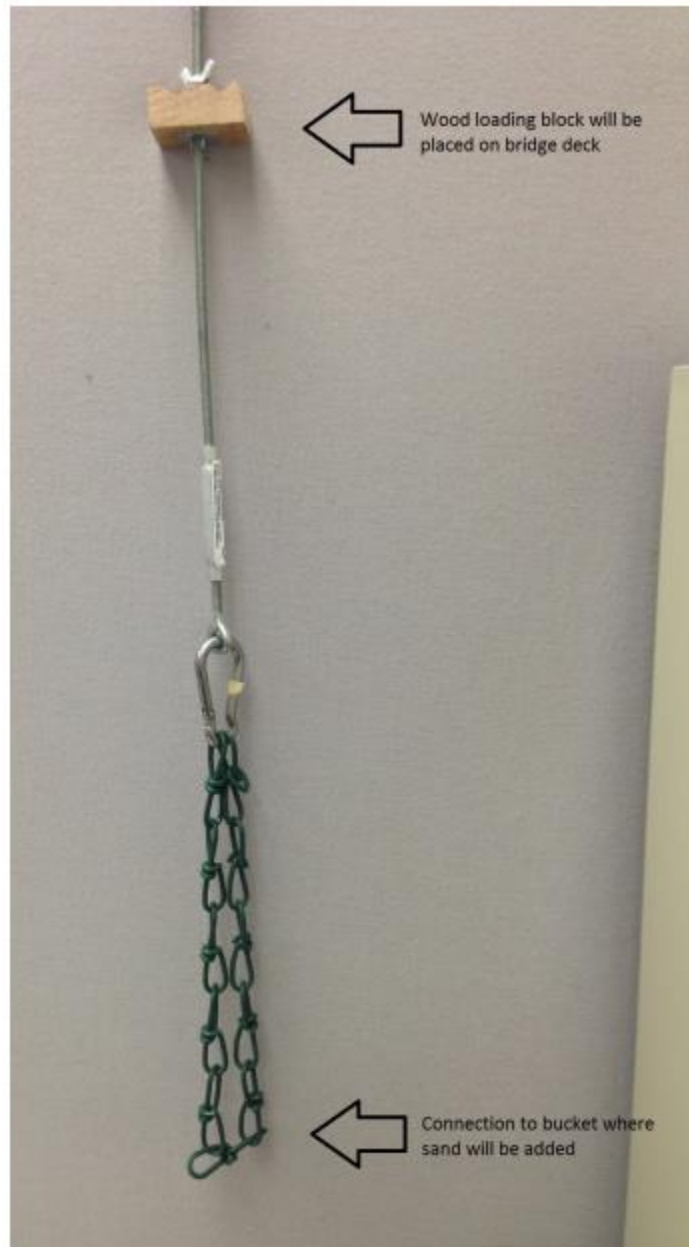
Figure 3 - Loading Block Connection
